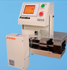
High performance NC clip feeder
